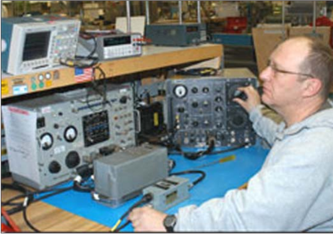
Bob Harvey, an electronics mechanic in Tobyhanna Army Depot's Avionics-Intelligence Electronics Warfare Systems Directorate, tests a TS-1843B/APX In-Flight Transponder Test Set. Tobyhanna technicians met an urgent request in January to repair and test four test sets to support Operation Iraqi Freedom.
