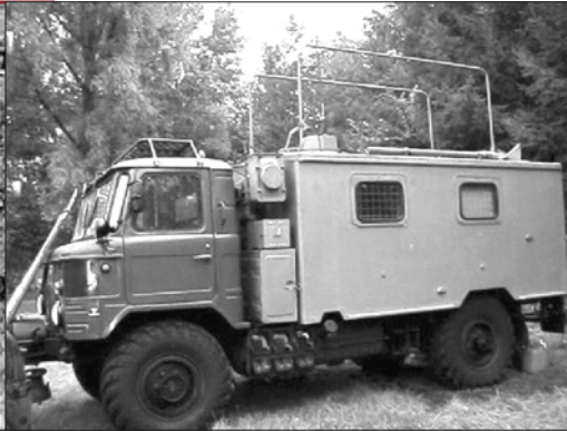
Fig. 9 (Left) A Russian communications vehicle with two vertical loop elements.
