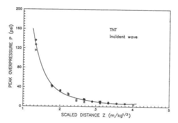
Figure 7. Overpressure as a function of scaled distance in incident-wave region for TNT ( $\sim 11.3$  kg).
