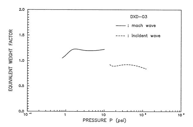
Figure 9. TNT-equivalent weight factor of DXD-03.
