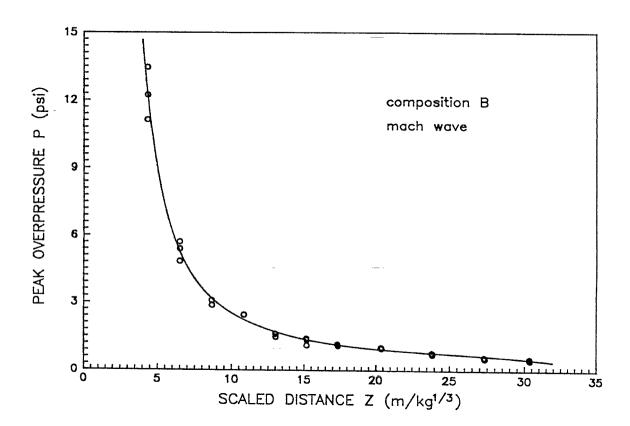
Figure 6. Overpressure as a function of scaled distance in Mach-wave region for composition B ( $\sim 12.3$  kg).
