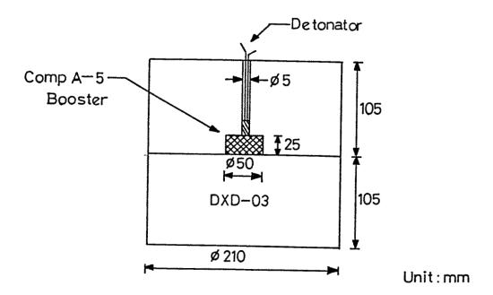
Figure 1. Configuration of a DXD-03 charge ( $\sim$  13 kg).
