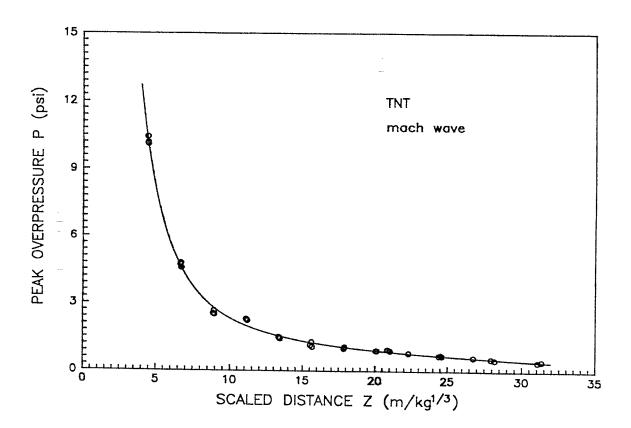
Figure 8. Overpressure as a function of scaled distance in Mach-wave region for TNT ( $\sim 11.3$  kg).
