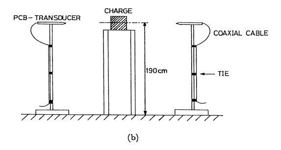
Figure 2. Experimental setup of blast-effect test; (a) gauge location and (b) height of a DXD-03 charge and gauges.
