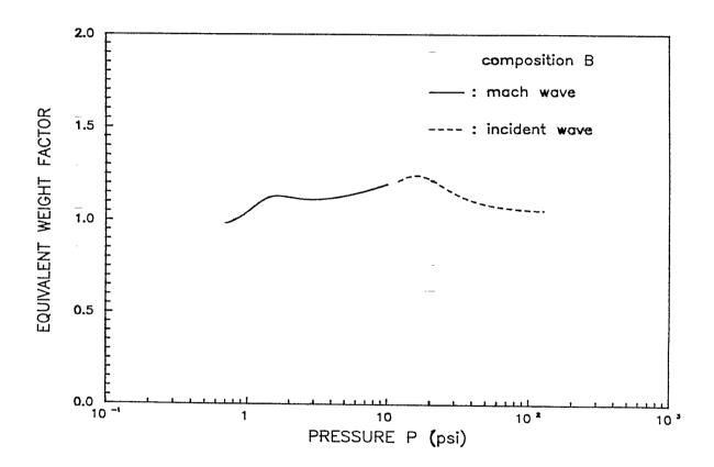
Figure 10. TNT-equivalent weight factor of composition B.
