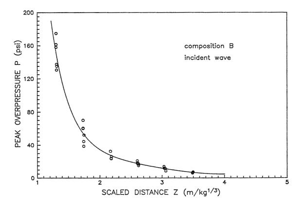
Figure 5. Overpressure as a function of scaled distance in incident-wave region for composition B ( $\sim 12.3$  kg).
