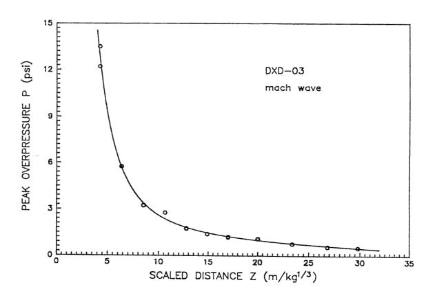
Figure 4. Overpressure as a function of scaled distance in Mach-wave region for DXD-03 ( $\sim 13$  kg).
