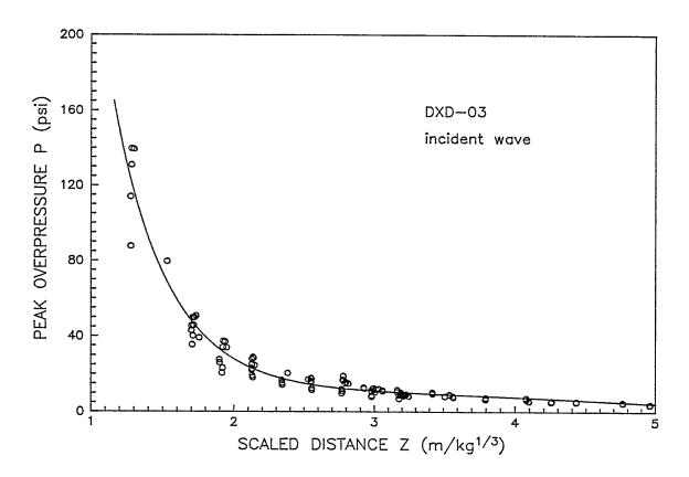
Figure 3. Overpressure as a function of scaled distance in incident-wave region for DXD-03 ( $\sim 13$  kg).
