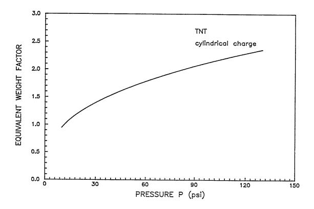
Figure 11. Geometry effect of cylindrical TNT charges (length/diameter = 1) over spherical charges.
