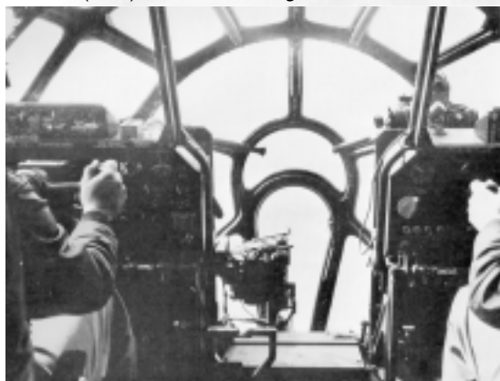
B-29 Superfortress bombers on their way to Japan. (Inset) A Norden bombsight in the nose of a B-29.
