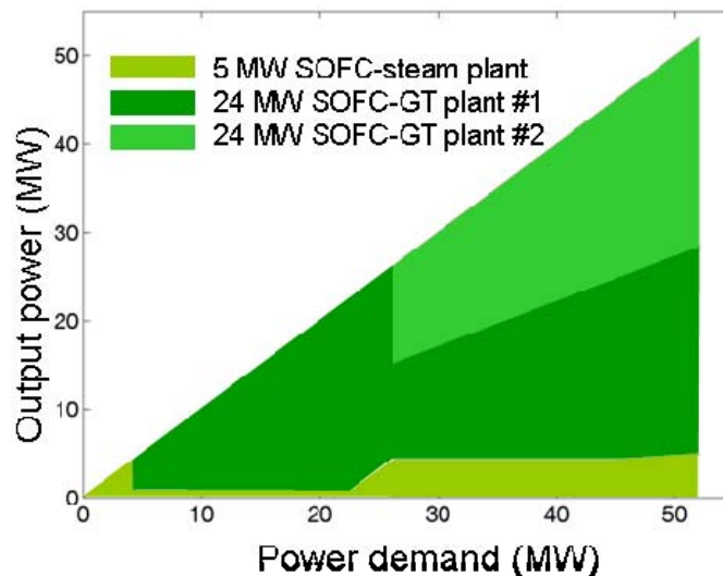
Figure 7: Power split among three SOFC power plants for any given power demand.
