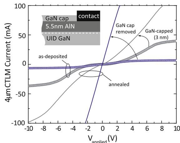
**Fig. 2.** Two-point current–voltage characteristics comparing contacts to 3 nm GaN-capped and removed GaN cap AlN/GaN for as-deposited and post-annealed metal. IV characteristics demonstrate the necessity to remove the 3 nm GaN cap in order to achieve a linear IV characteristic after annealing.
