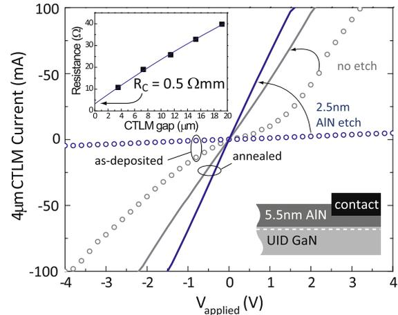
**Fig. 1.** Two-point current–voltage characteristics comparing the 2.5 nm pre-metallization etched and non-etched contacts to AlN/GaN for as-deposited and post-annealed metal. IV characteristics demonstrate the reduction in contact resistance due to the pre-metallization etch. Inset showing CTLM measurement and fit data for the lowest  $R_c$  value of  $0.5 \Omega \text{ mm}$  obtained through the pre-metallization etch.
