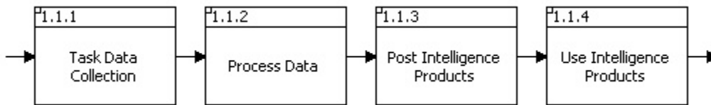
Figure 31. Provide Intelligence Operational Function FFBD.
