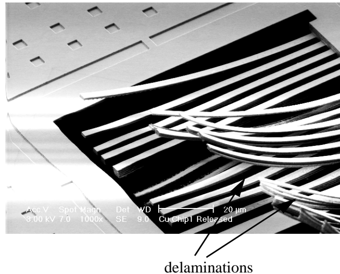
Figure. 5-8. Delamination of the mechanical structures with the post-CMOS Al- \text{SiO}_2 microstructure etch recipe. The extra fluoride in the low-K dielectric causes severe delamination.
