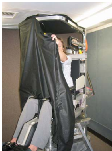
Figure 2. Rotating chair, showing adjustable head stops and visual canopy (being closed).
