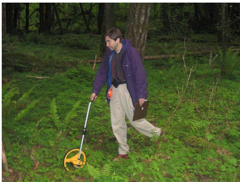
Figure 3-10. Measuring course length with measuring wheel.
