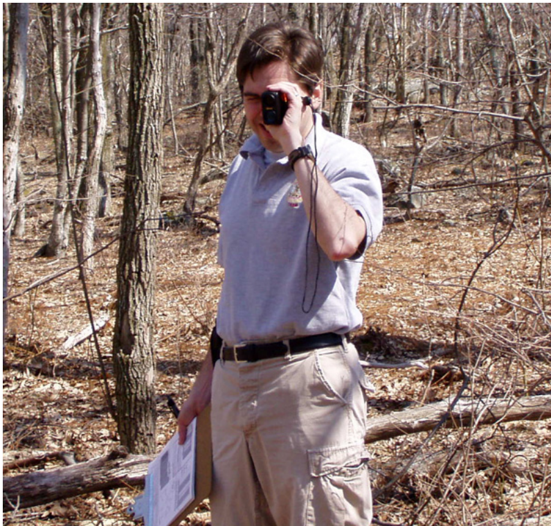
Figure 3-8. Hand-held Laser Range Finder in use.
