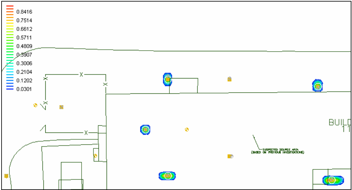
Figure E.8: MnO_4^- Distribution, 5gpm, 1.0mg/mL KMnO_4 , Layer 2, fast NOD present
