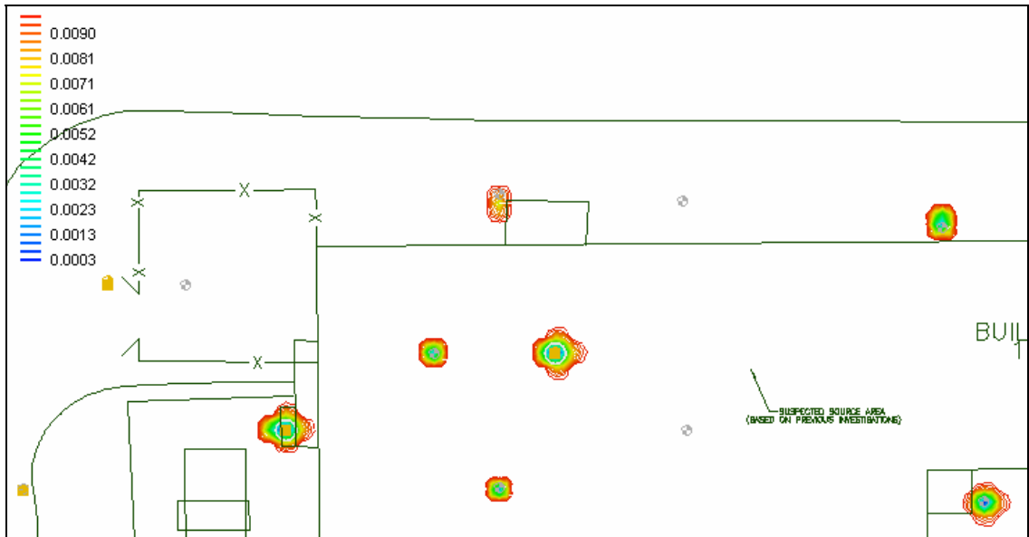
Figure E.54: Fast NOD Distribution, 10gpm, 0.25mg/mL KMnO 4 , Layer 3
