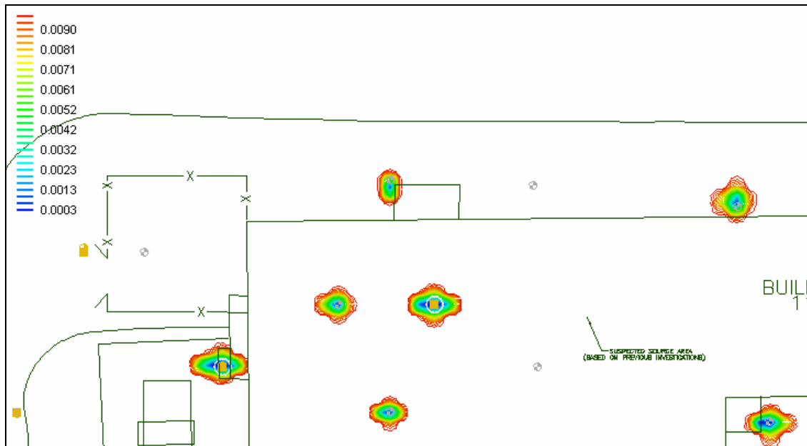
Figure E.56: Fast NOD Distribution, 5gpm, 1.0mg/mL KMnO 4 , Layer 3
