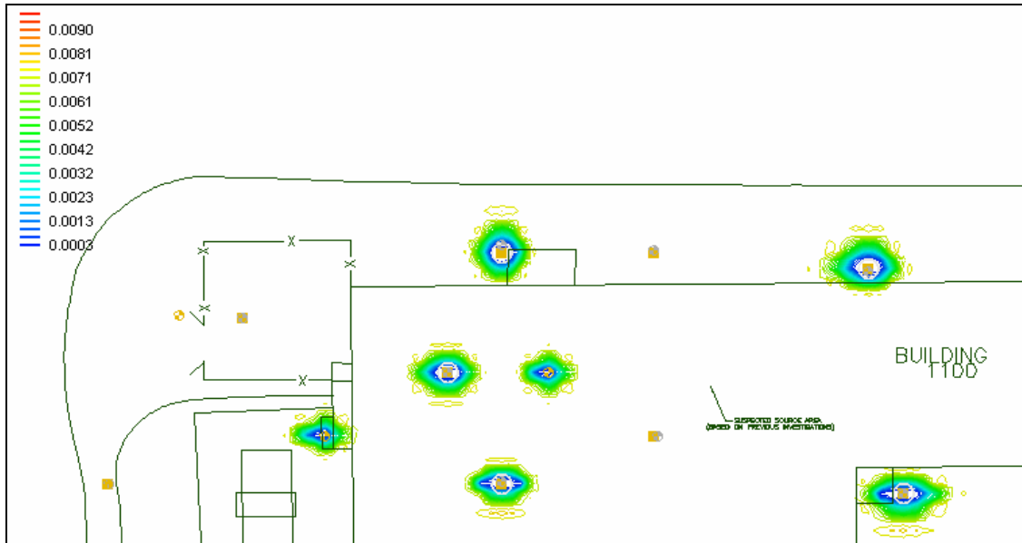
Figure E.43: Fast NOD Distribution, 15gpm, 1.0mg/mL KMnO 4 , Layer 2
