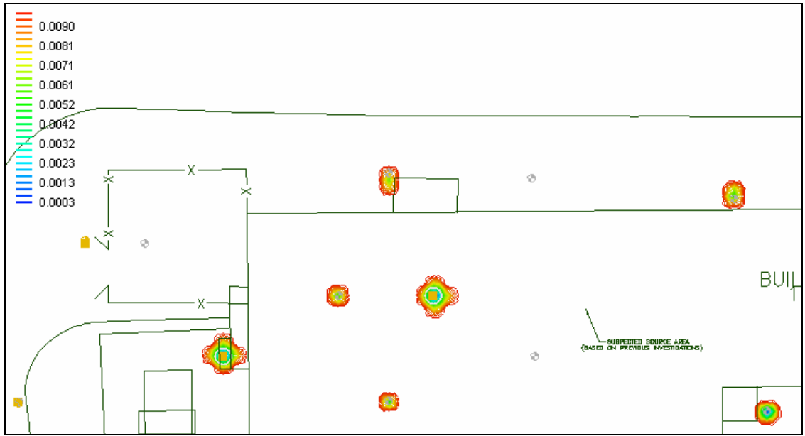
Figure E.53: Fast NOD Distribution, 8gpm, 0.25mg/mL KMnO 4 , Layer 3
