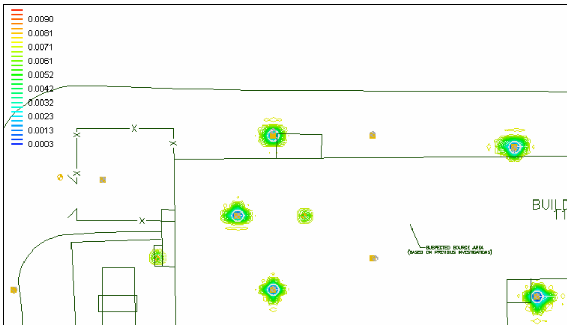
Figure E.48: Fast NOD Distribution, 8gpm, 0.25mg/mL KMnO 4 , Layer 2, fast NOD present (decreased k)
