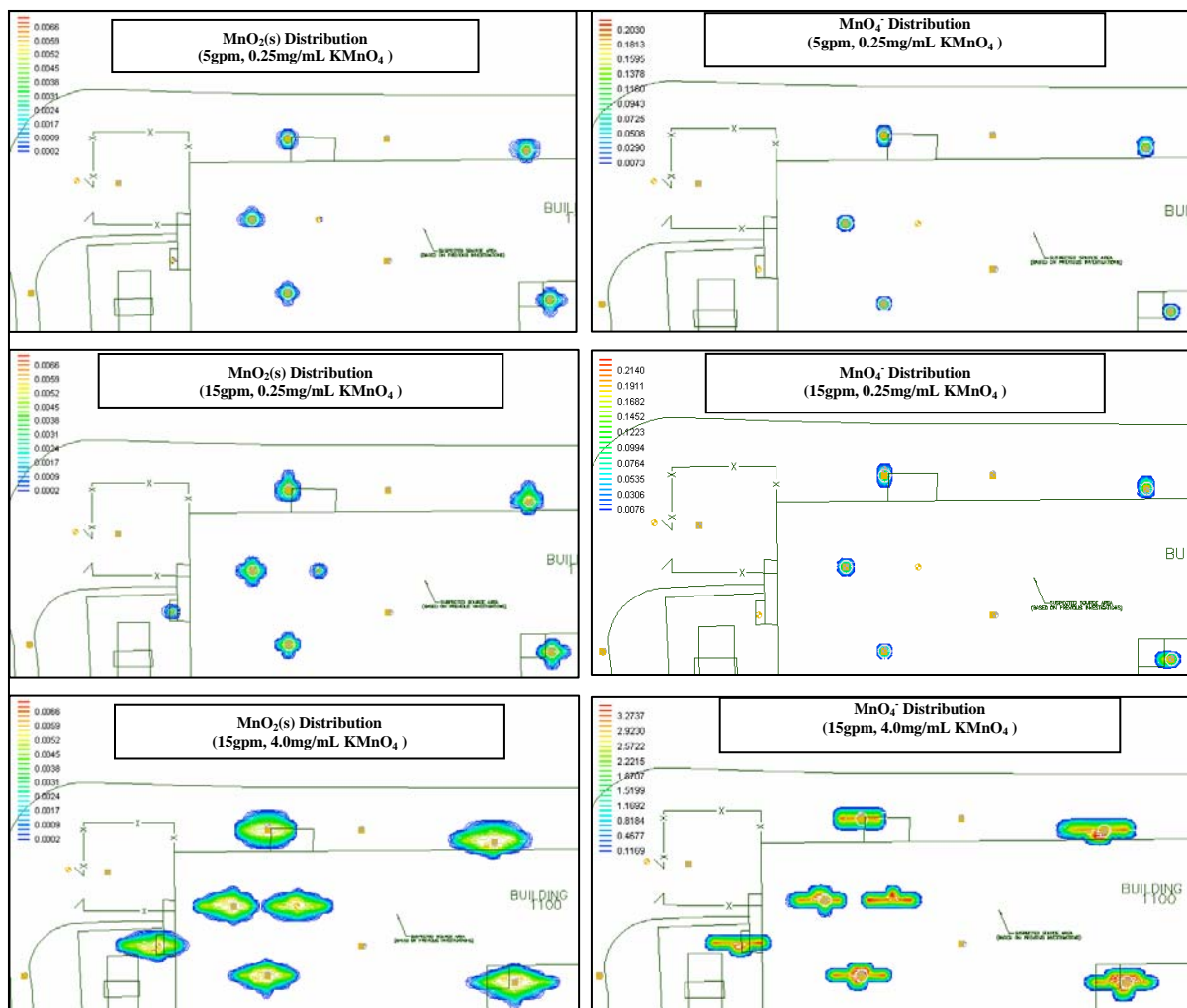
Figure 5.5: Comparison of Oxidant Transport at NTC Site, \text{MnO}_2(\text{s}) (left), \text{MnO}_4^- (right) (middle row-base case, top-low flow rate, bottom-high oxidant concentration)
