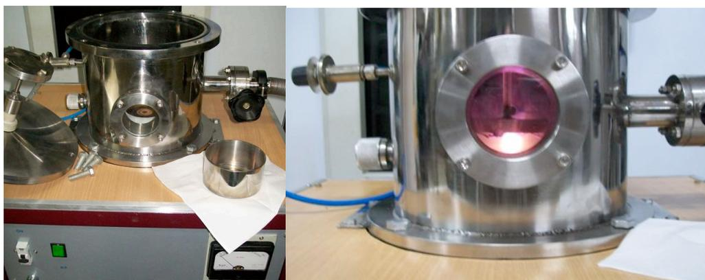
Figure: (left) Chamber with power supply. Substrate holder is to the left. (right) Chamber in operation with Cu deposition.
