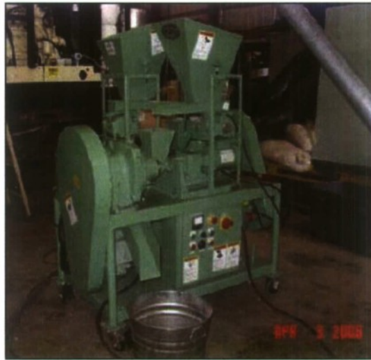
Figure 5. Two High Capacity Laboratory Pelletizers Mounted on a Single Table with Casters
