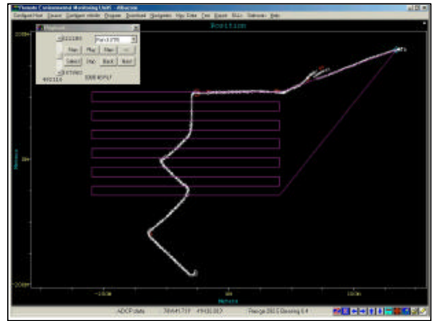
Figure 10. AMP continues directing for ~3 minutes and then relinquishes control back to the REMUS computer. The REMUS computer's 1 st objective is to return to the initial breakoff point.
