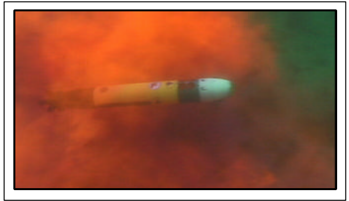
Figure 21. REMUS vehicle swimming through dye plume.
