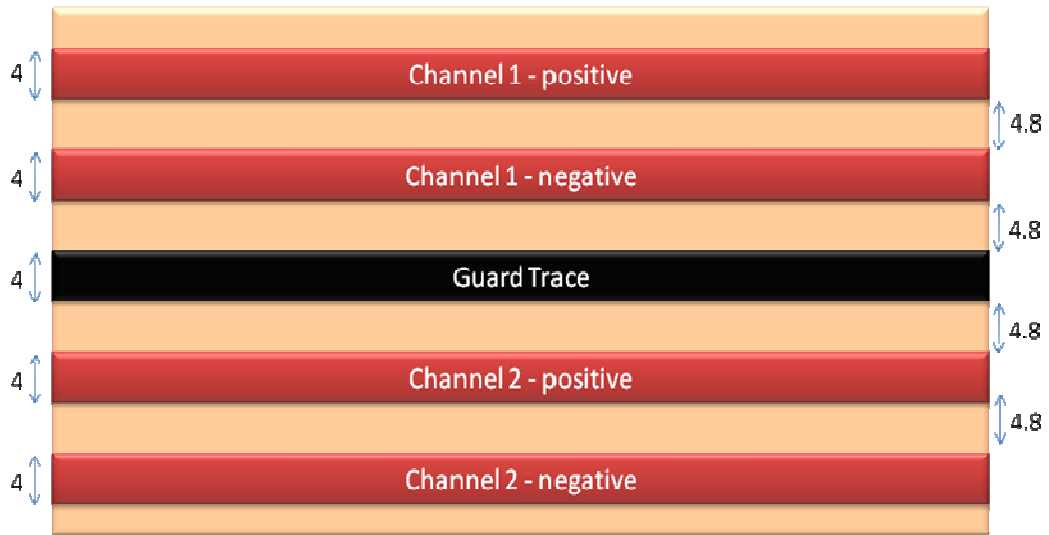
Figure 3.9 - Guard Trace, each differential pair is separated from its neighbors by a properly terminated guard trace
