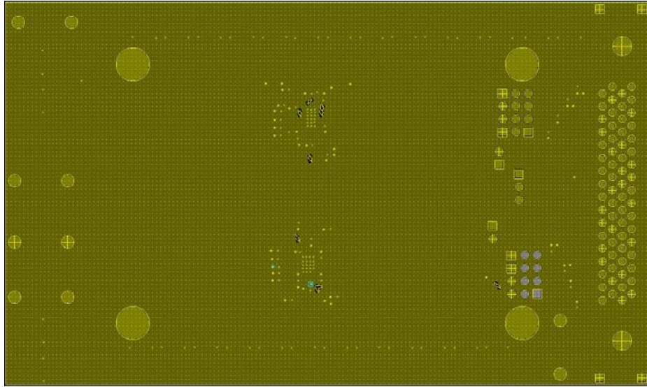
Figure 3.14 - Ground Layer was designed to provide the cleanest return path to the high speed signals routed above.
