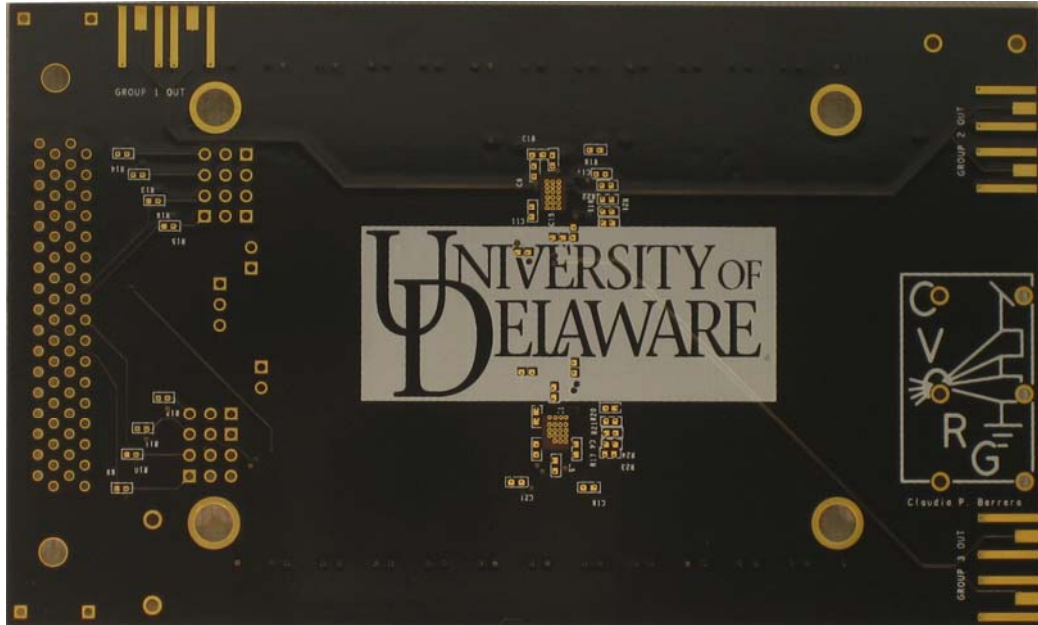
Figure 3.17 - PCB Bottom Layer
