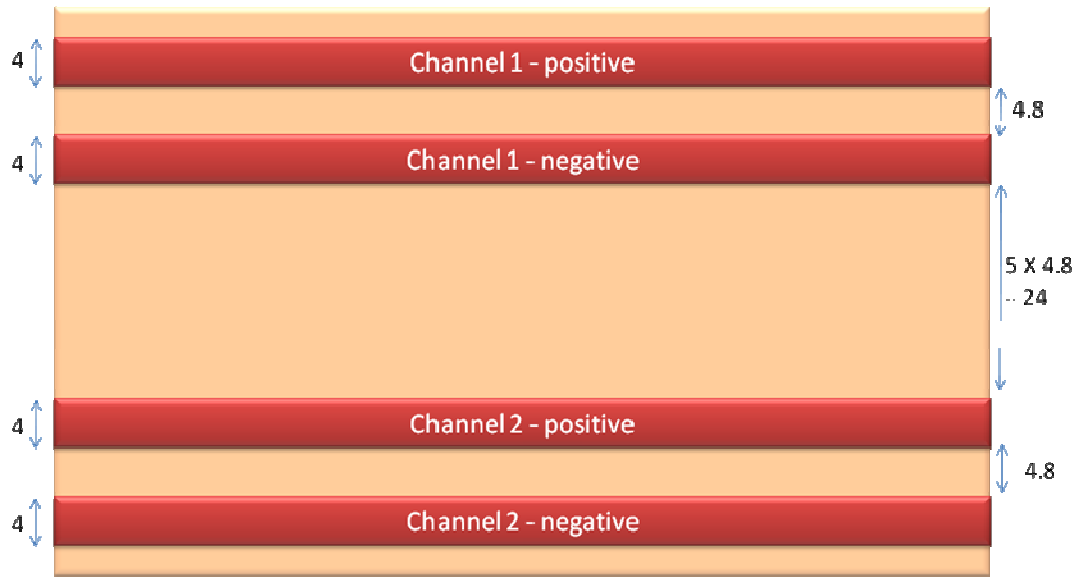
Figure 3.8 - Rule of Thumbs, each differential pair is separated from its neighbors five times the minimum spacing
