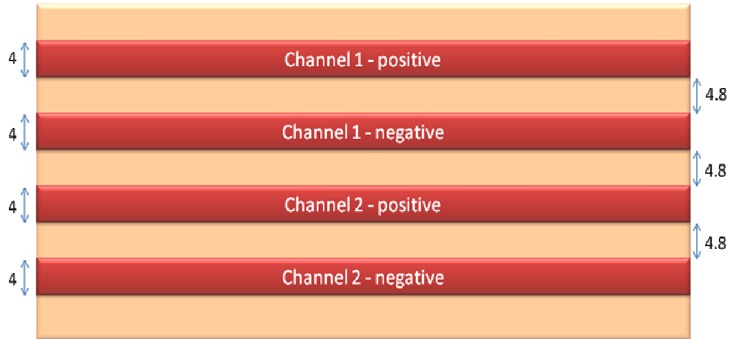
Figure 3.10 - Minimum spacing between channels. The distance between channels is the minimum allowed by the manufacturer.
