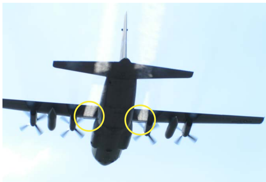
The fuselage-mounted spray booms (circled) on a USAF C130H airplane are shown in operation during evaluation flights at the Air Force Range, Avon Park, Florida.
