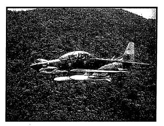
an advertised range of nearly 3000 miles. The hardened canopy can withstand a birdstrike up to 270kts. The two-seat version has an advertised endurance of over four hours with a standard weapon loadout. A single seat version offers an additional 80
