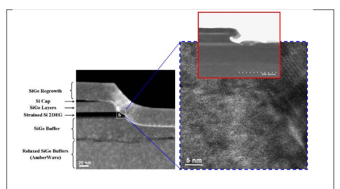
Fig. 1. TEM micrograph of and edge after SiGe regrowth. In the red inset we show an example of non-conformal regrowth from previous years.
