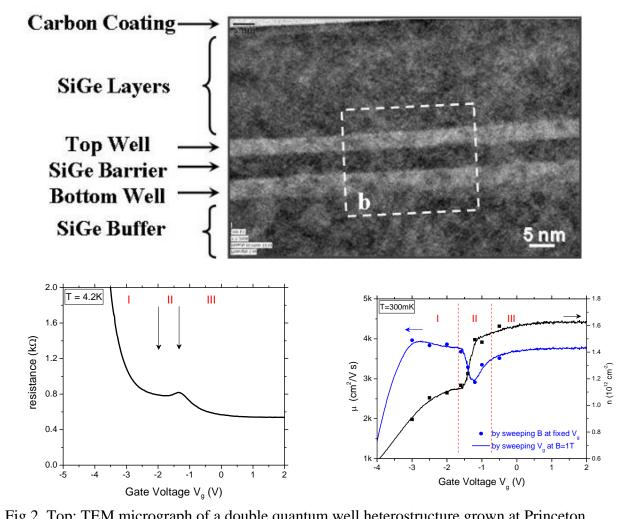
Fig 2. Top: TEM micrograph of a double quantum well heterostructure grown at Princeton. Bottom: resistance, mobility and electron density of the DQW as a function of the top gate voltage. Peak in resistance (and corresponding dip in mobility) corresponds to the depletion of the top well and transfer of the electron density into the bottom one.
