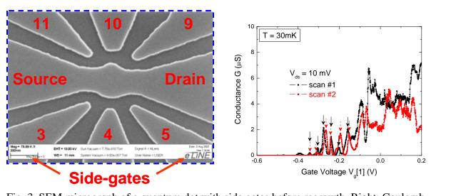
Fig. 3. SEM micrograph of a quantum dot with side gates before regrowth. Right: Coulomb blockade measured at 30 mK as a function of voltage on the plunger gates 4 and 10. The shift of CB peaks is attributed to the spurious charging effects at the interface.
