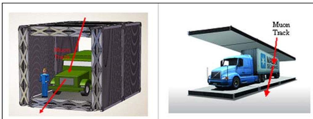
Figure 13. Schematic Drawing of Muon Tomography Inspection Station Configurations: Tunnel and Top/Bottom
