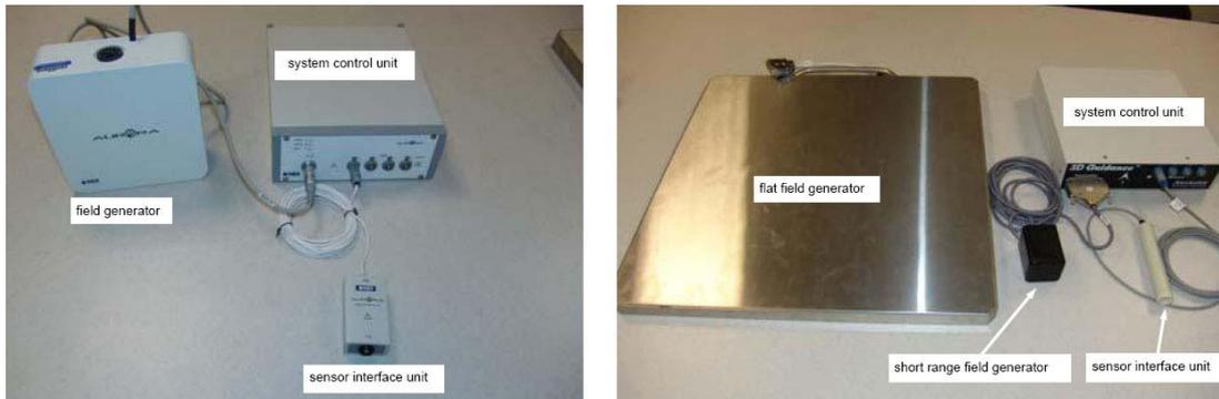
**Figure 9: Electromagnetic tracking systems and their components used in this study (left) Aurora and (right) 3D Guidance**
