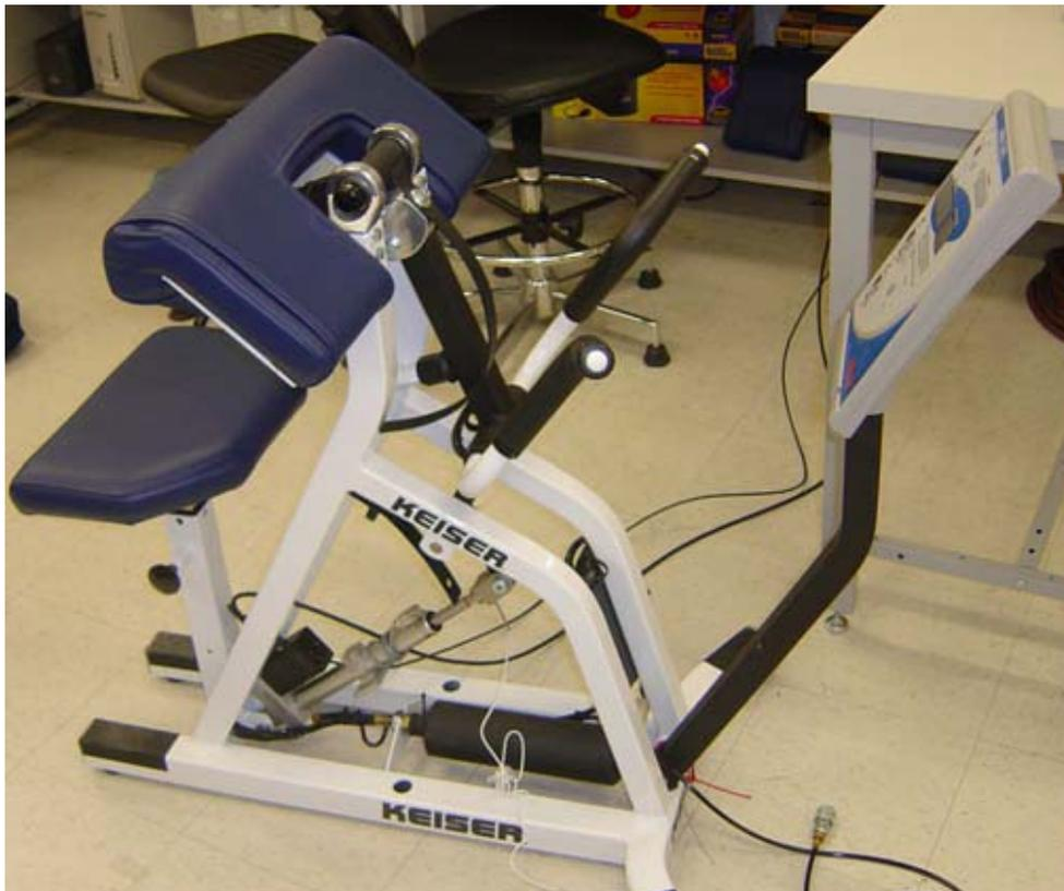
**Figure 5: Keiser Arm Curl 250 retrofitted with UltraMotion actuator**
