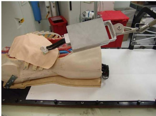
Fig 8. Robot assisted needle placement phantom study.
