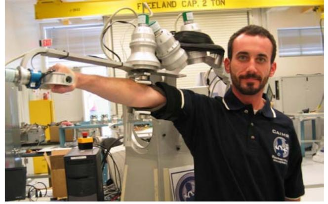
Fig. 5. Exoskeleton shown at 90° shoulder abduction.
