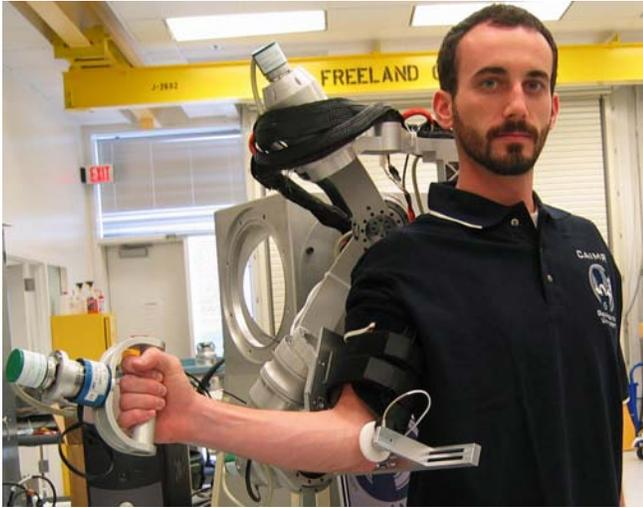
Fig. 4. Exoskeleton shown performing external/internal rotation at about 90° elbow flexion.
