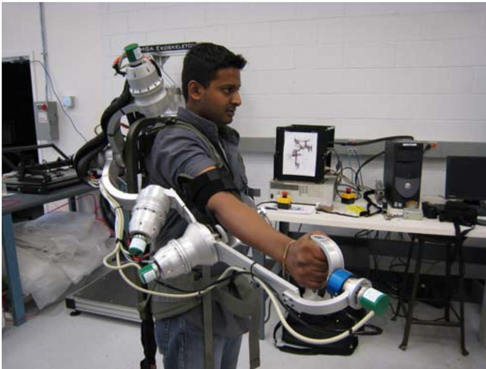
**Figure 4: The MGA Exoskeleton has five powered joints including a three-axis intersecting shoulder and a scapula elevation joint**
