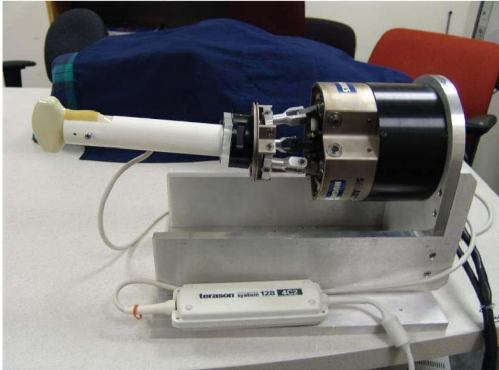
**Figure 1: Parallel mechanism robotic device holding ultrasound probe**
