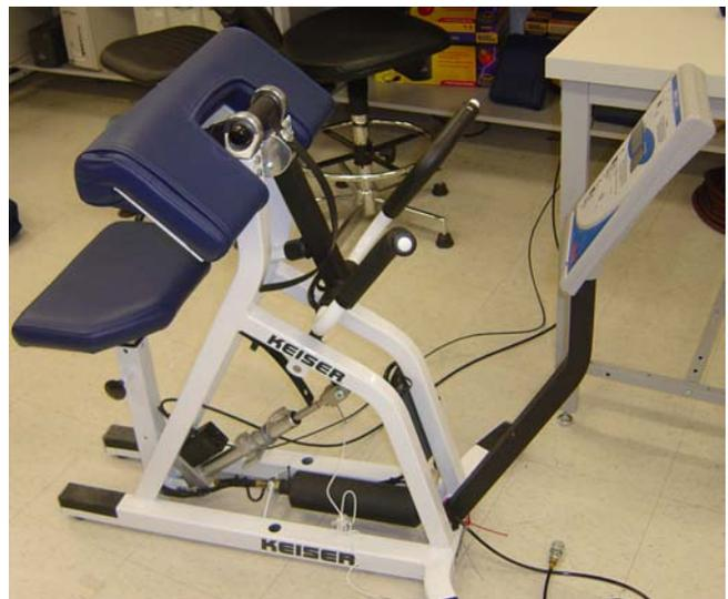
Fig. 1. Keiser Arm Curl 250 retrofitted with UltraMotion actuator.
