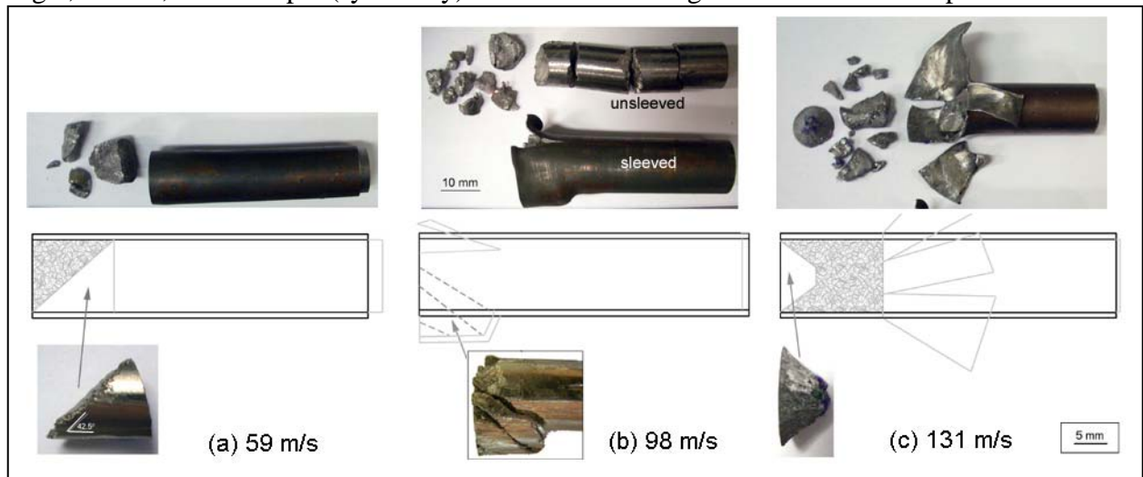
Fig. 5. Monolithic BMG rods (confined by stainless steel sleeves) recovered post-impact after anvil-on-rod dynamic compression tests performed at (a) 59 m/s, (b) 98 m/s, and (c) 131 m/s.
