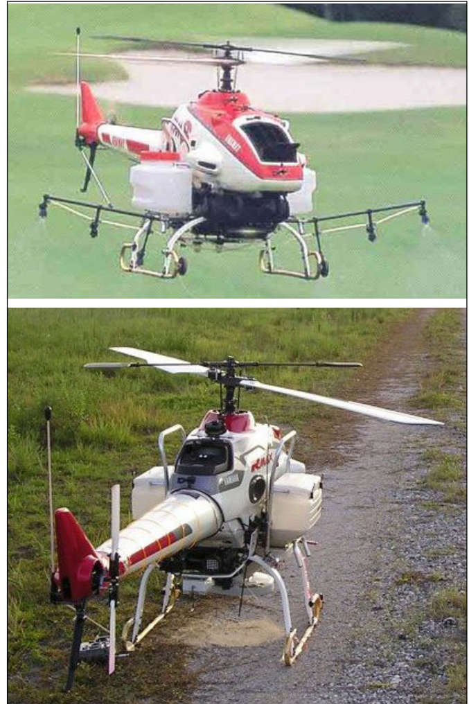
Figure 1. Yamaha RMax unmanned aerial vehicle fitted with ULV spray nozzles (top) and with twin hopper (bottom) for application of granular larvicide to control mosquitoes.
