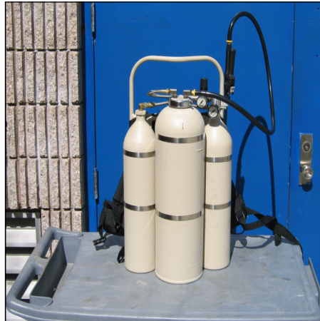
Figure 2. The first backpack ULV sprayer system developed under DWFP grants operates almost silently with compressed air from cylinders.
