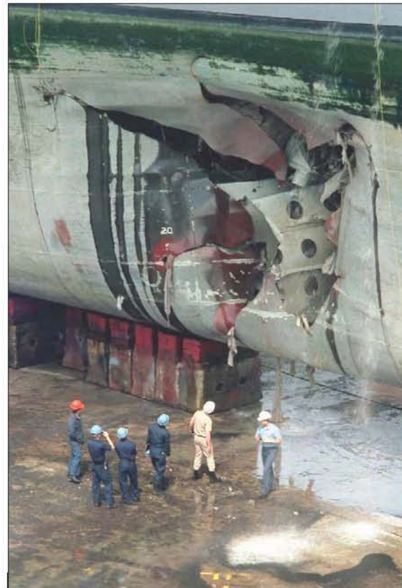
Mine damage to USS TRIPOLI after hitting a mine during the first Persian Gulf War in February 1991
