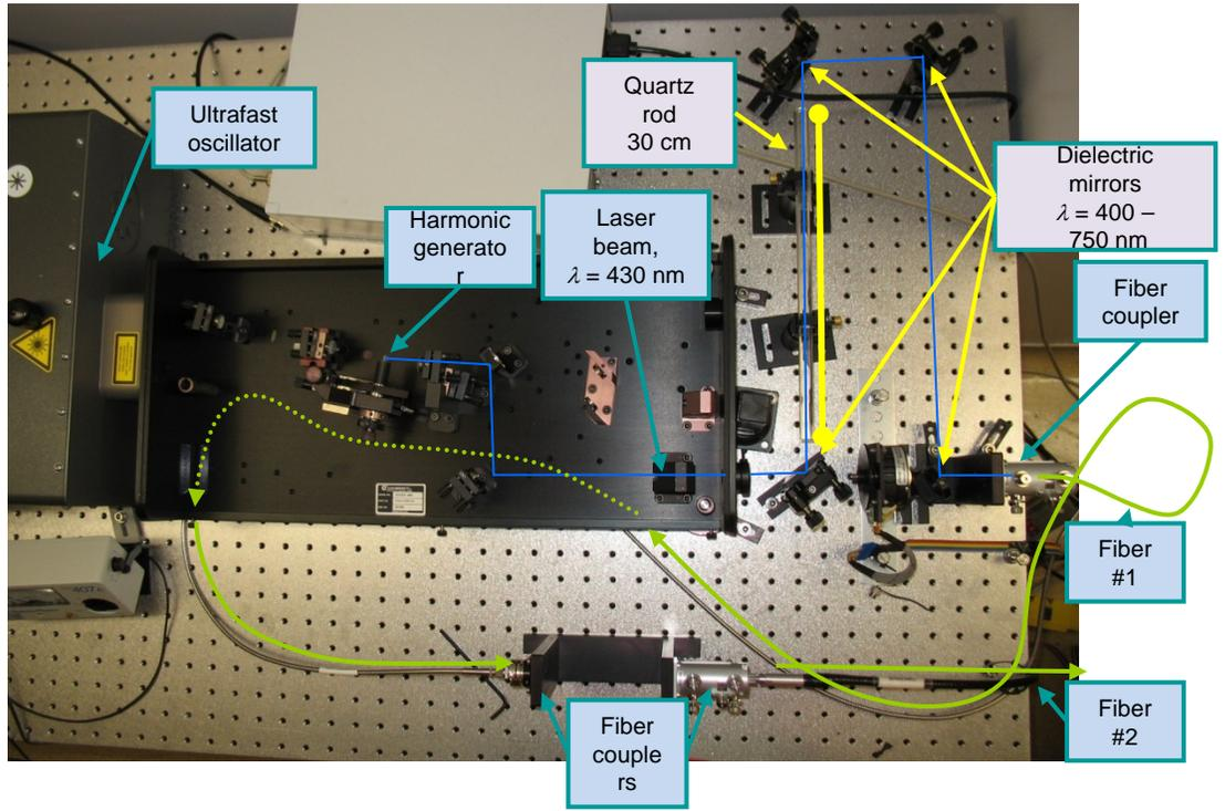
**Figure 20:** Addition of pulse stretcher to FLIM system
