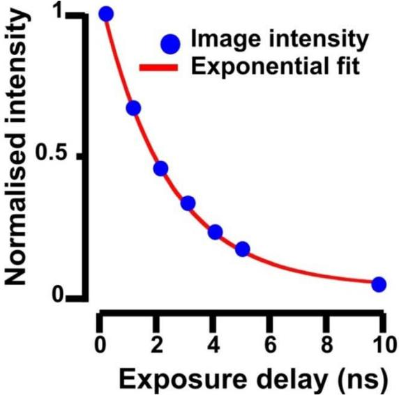
High speed data acquisition from 7 points provides an accurate estimation of FLIM. We have extended this to two measurements with custom gates and the resulting FLIM estimates are acceptable and can be acquired fast enough for screening (0.5 seconds).
