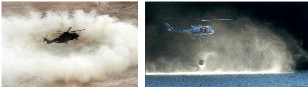
Figure 1: The picture on the left illustrates how rotor wash can blow sand upward and then force it down through the rotors over the windscreen, thereby creating a "brownout" that blocks the pilots outside view. The picture on right provides an example of how a similar situation happens when hovering over water.
