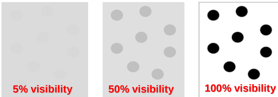
Figure 7: Appearance of VVSD surround dot pattern when viewed through the variable contrast stimulus device. The image on the left represents near maximum gray saturation and the image to the right indicates a condition of zero saturation.
