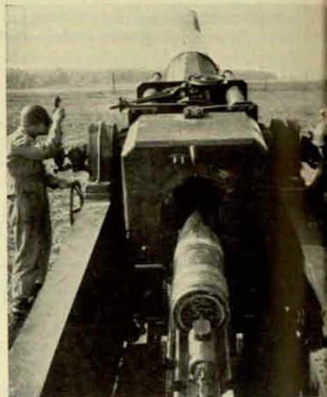
Rear view of the 280. The hydraulic power rammer is pushing a shell into the breech. After the powder charge is rammed home the loading track is moved out of the way. The soldier at the left is peering through the sight of the big gun.
