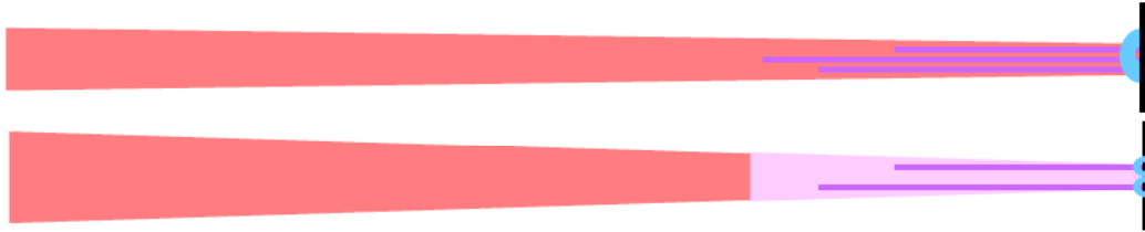
FIGURE 16: Schematic diagram of potential shock wave geometries that can result from the interaction of filamenting laser pulses with a target.
