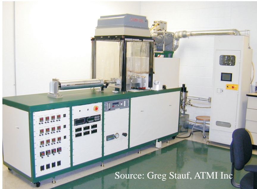
Figure 3.4: MOCVD chamber at ATMI, Inc.
