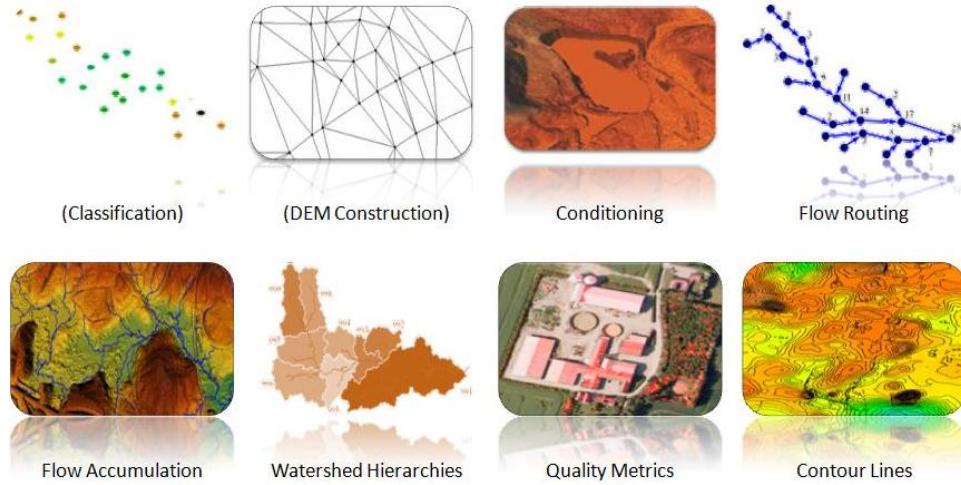
Figure 1. Various stages in our pipeline constructed on the Neuse river basin: (a) LIDAR data (500M points), (b) grid DEM at 10ft resolution, (c) flow network, (d) watershed hierarchy.
