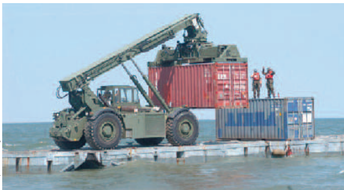
Naval Amphibious Construction Battalion Two discharging containers across the beach from a causeway ferry during Joint Logistics Over-The-Shore (JLOTS) 2006, a multi-service cargo distribution exercise. JLOTS operations discharge strategic vessels without the benefit of a fixed port. SDDC provided the JLOTS 2006 joint task force commander.
