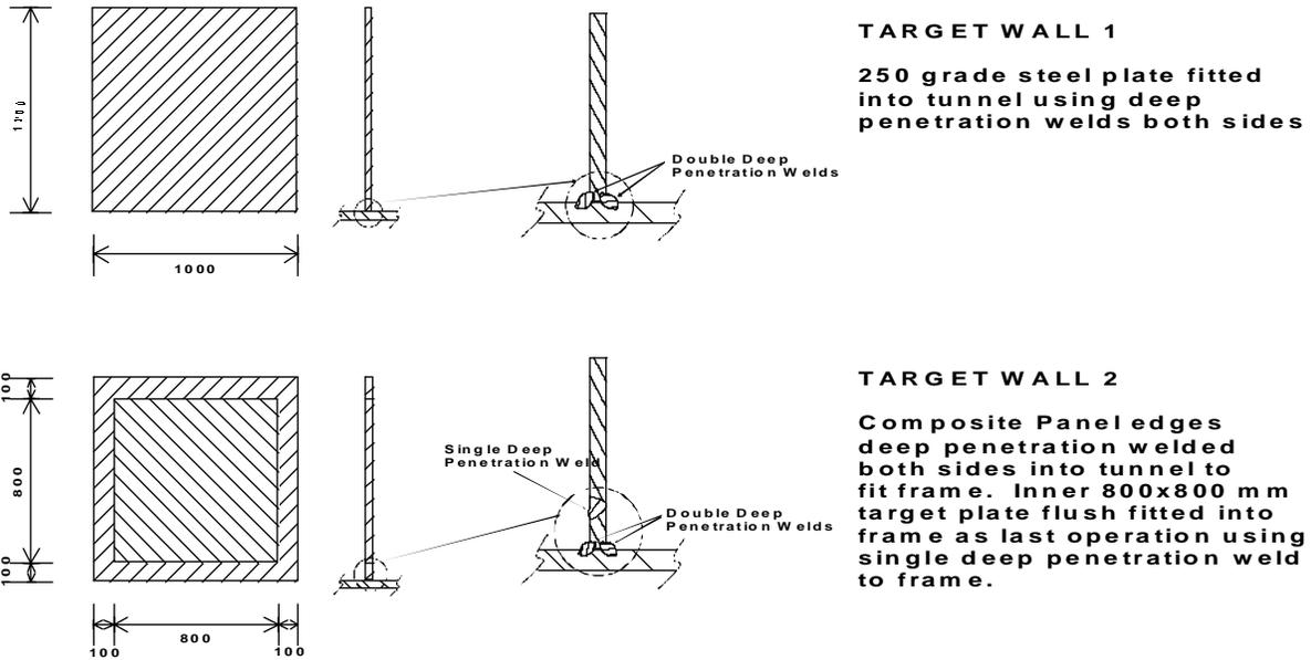
**Figure 1c. Test panel construction and fitment details.**
