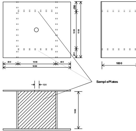
**Figure 1b. Construction details of the blast test rig.**
