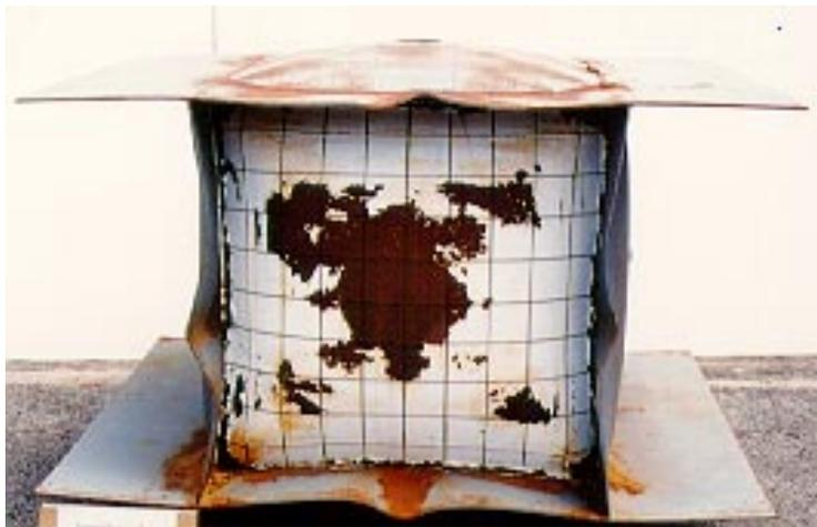
**Figure 2. Deformation of test rig and 5mm test panel for 1000g Pentolite Charge.**
