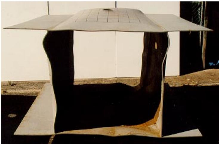
**Figure 6. Deformation and failure of 2.5 mm sample panels for 1000g Pentolite Charge.**
