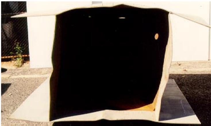
**Figure 5. Deformation and failure of 3mm sample panel for 1000g Pentolite Charge.**
