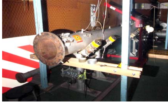
Fig. Air driven shock tube at the WRAIR/NMRC used for blast pressure wave generation.
