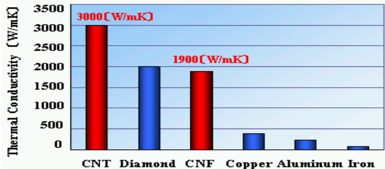
Fig. 3. Thermal conductivity of CNTs and other materials
