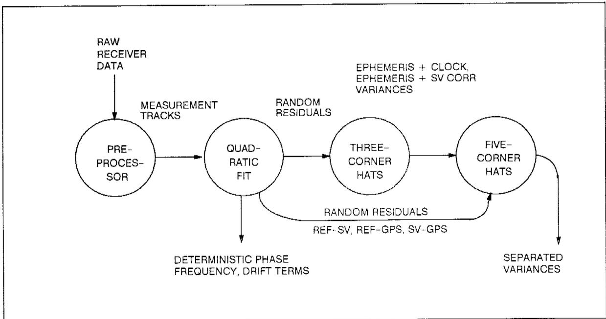
**Figure 11.** Data flow shows procedure for multicorner hat.
