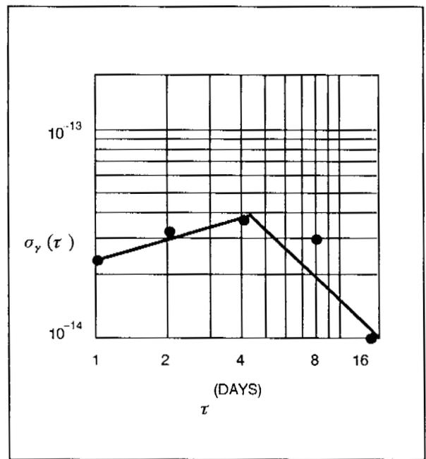
**Figure 6.** An HP 5061B cesium at Interstate exhibits excellent smoothed frequency stability versus UTC (USNO).
