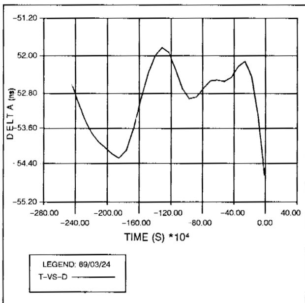
**Figure 7.** Common-view weighted mean error shows 0.7-nsec deviation.
