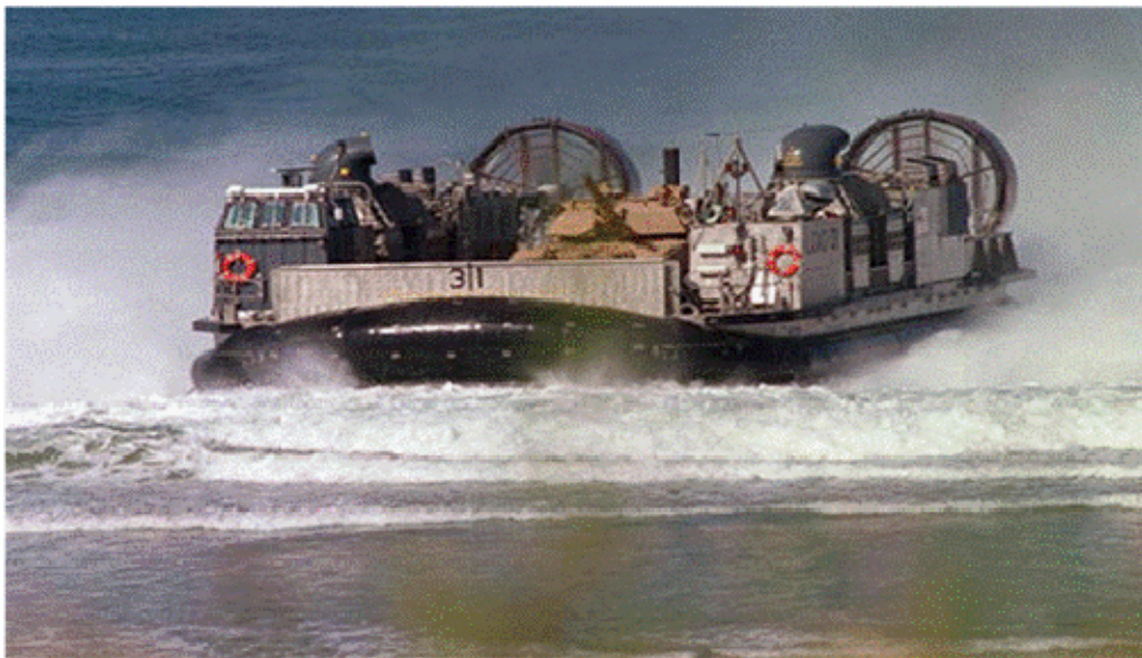
Figure 3. Landing Craft Air Cushion (LCAC) at 75-Ton Overload. (From 18 )
