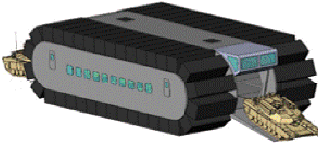
Figure 4. Conceptual Depiction of Ultra Heavy-lift Amphibious Connector (UHAC). (From 28 )
