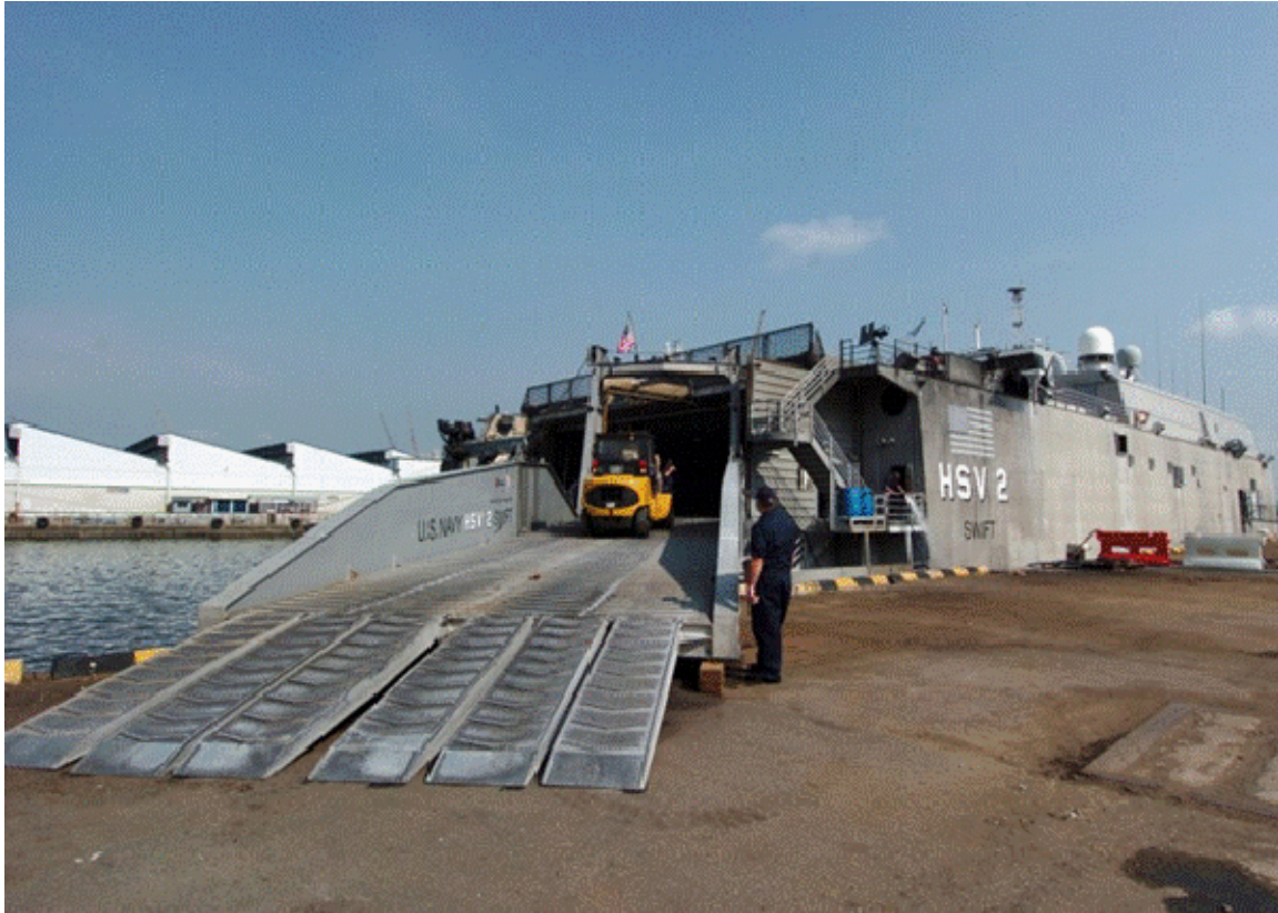
Figure 14. JHSV Offloading Cargo to Pier. (From 68 )
