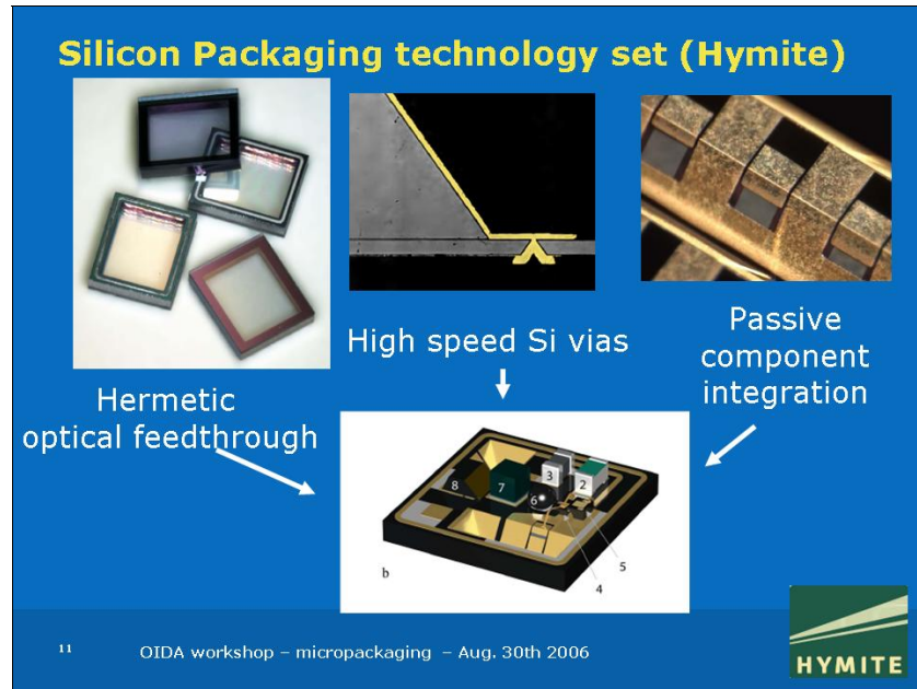
Figure 23: High speed signaling via in the silicon wafer package approach (Courtesy of Intel: M. Finot)
