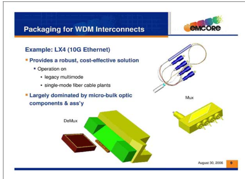
Figure 12: Plastic molded optics for coupling in single or multimode LX4 applications (Courtesy of EMCORE: K. Jackson)
