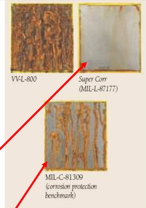
FIGURE 2: A second round of tests determined that the lubricating and corrosion protection properties of Super Corr were superior to the product being used by the P-3 squadron at NADEP Jacksonville.
