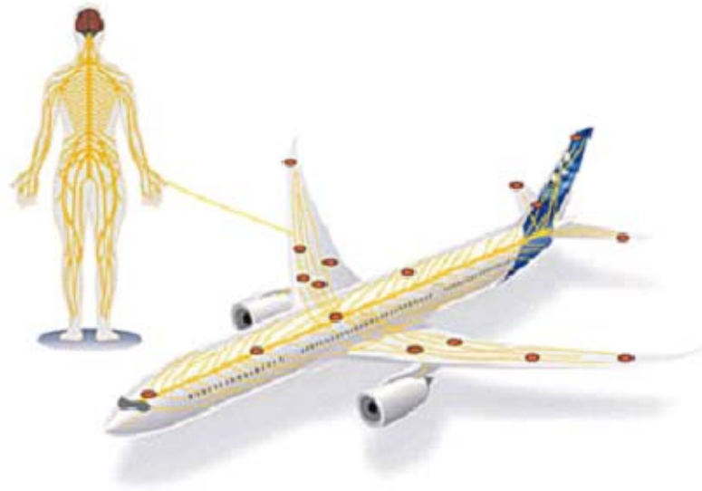
Figure 1. A Conceptual Illustration of Structural Health Monitoring [From 2].
