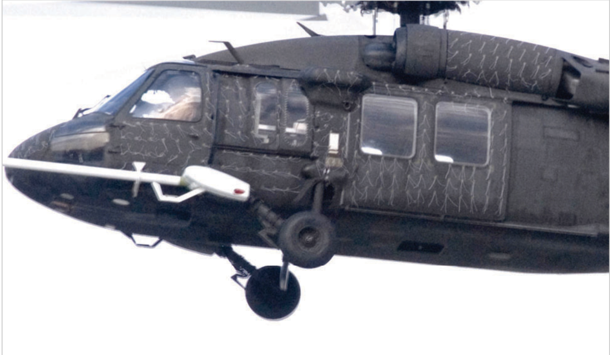
Figure 4(d). Overlay of three instantaneous airframe tuft images; Wheel height=50 ft.
