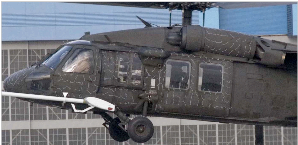
Figure 5(b). Single instantaneous airframe tuft pattern; Wheel height=5 ft.
