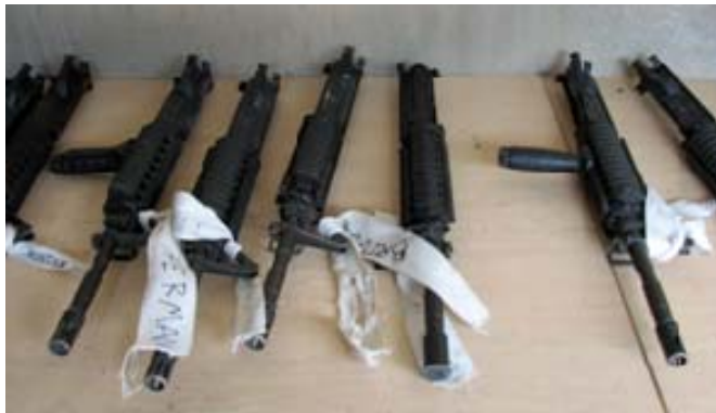
Figure 21. Barrel replacement with the M16-A2 is required to accommodate SESAMS rounds.
