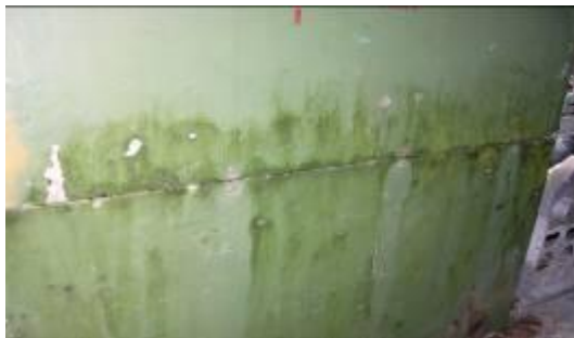
Mildew Growth Inside T-39 Aircraft Before Cleaning
