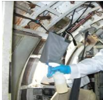
Cleaning Mildew Growth by Spraying Mildew Remover
