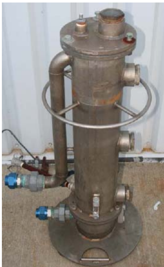
Figure 1: 20 gpm Vertical Canister Filter Separator
