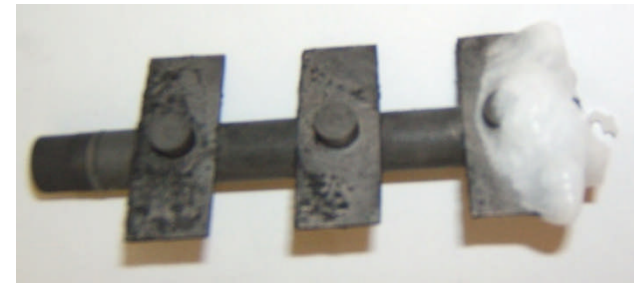
Graphite central rod with samples removed from corrosion cell
