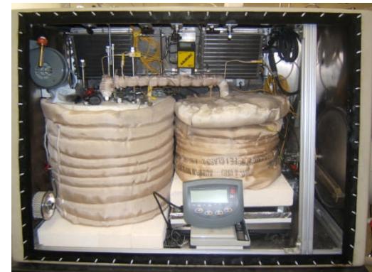
Salt transfer apparatus in glove-box
