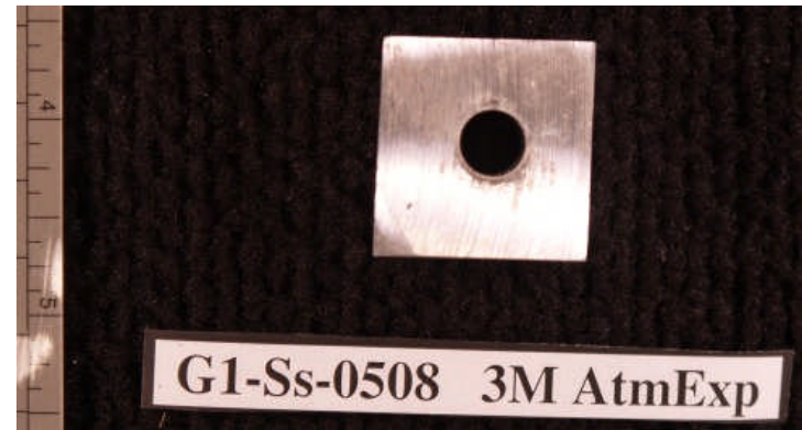
Slight discoloration on Al backside that was mated with the stainless steel
