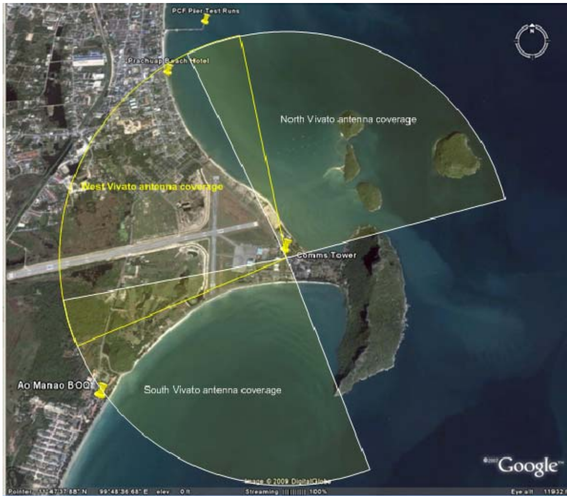
Figure 12. 802.11g wireless coverage sectors by Vivato antennas mounted on Comms Tower. (From Google Earth)
