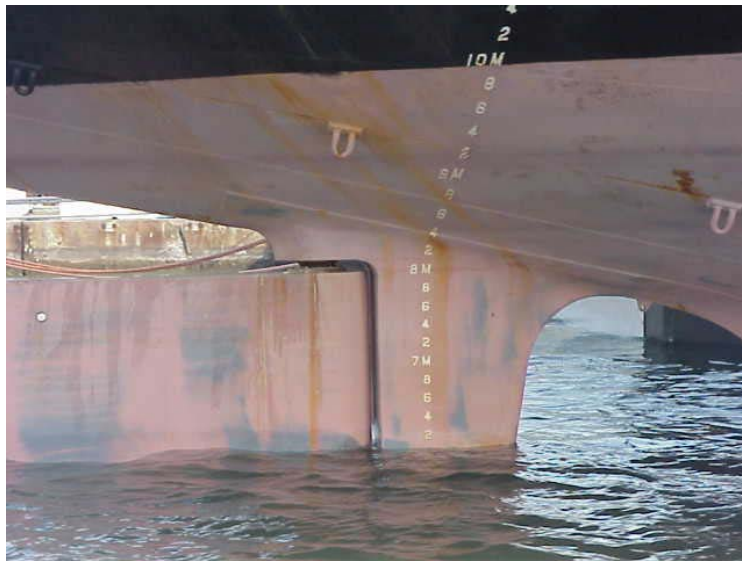
Figure 7. Example of aft draft marks on commercial tanker (From Guldner, 2002)
