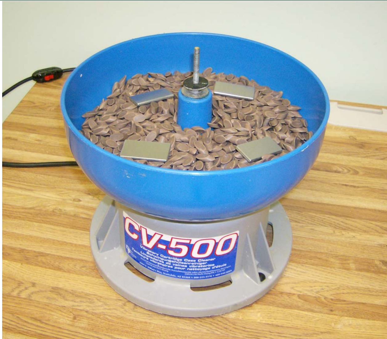
Small vibratory bowl with 0.28 m inner diameter filled with 4 kg of large ceramic media.
