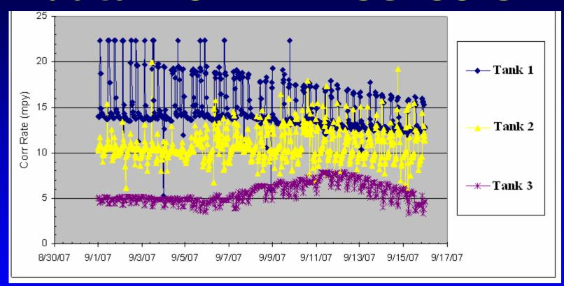
A wide variation in general corrosion rates was observed. The lowest rate consistent occurred in one of the water storage tanks at the site. The highest rate occurred at a pressure reducing valve with intermittent flow.
