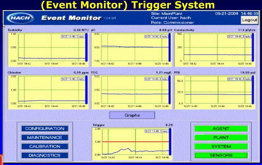
View all measurements and trigger signal from the main screen.
