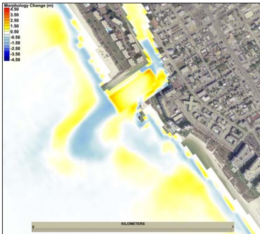
Figure 12. Modeled morphology change at Blind Pass for a dredged cut (alternative 1 for Blind Pass). Deposition within the dredged channel reached approximately 21,000 cubic meters after one year.
