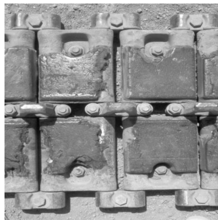
Figure 1B: Bushing failure (excessive gap between track blocks) led to track being "thrown"
