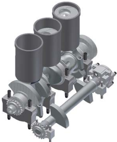
Figure 2: Crankcase Components including Oil Pump/Balancing Shaft
